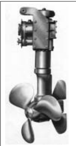
Rudderpropellers in pull and push version
