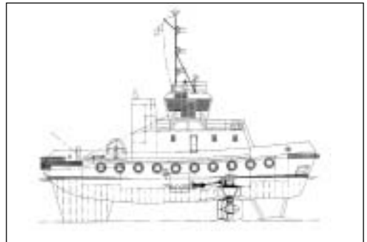
Tractor tug (Rudderpropellers in the front third of the tug)
